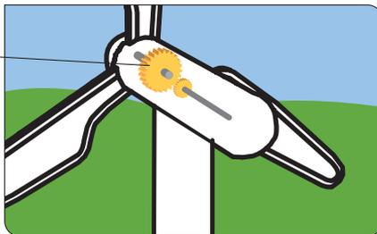
3. The gears turn a machine called a generator, which makes electricity.
